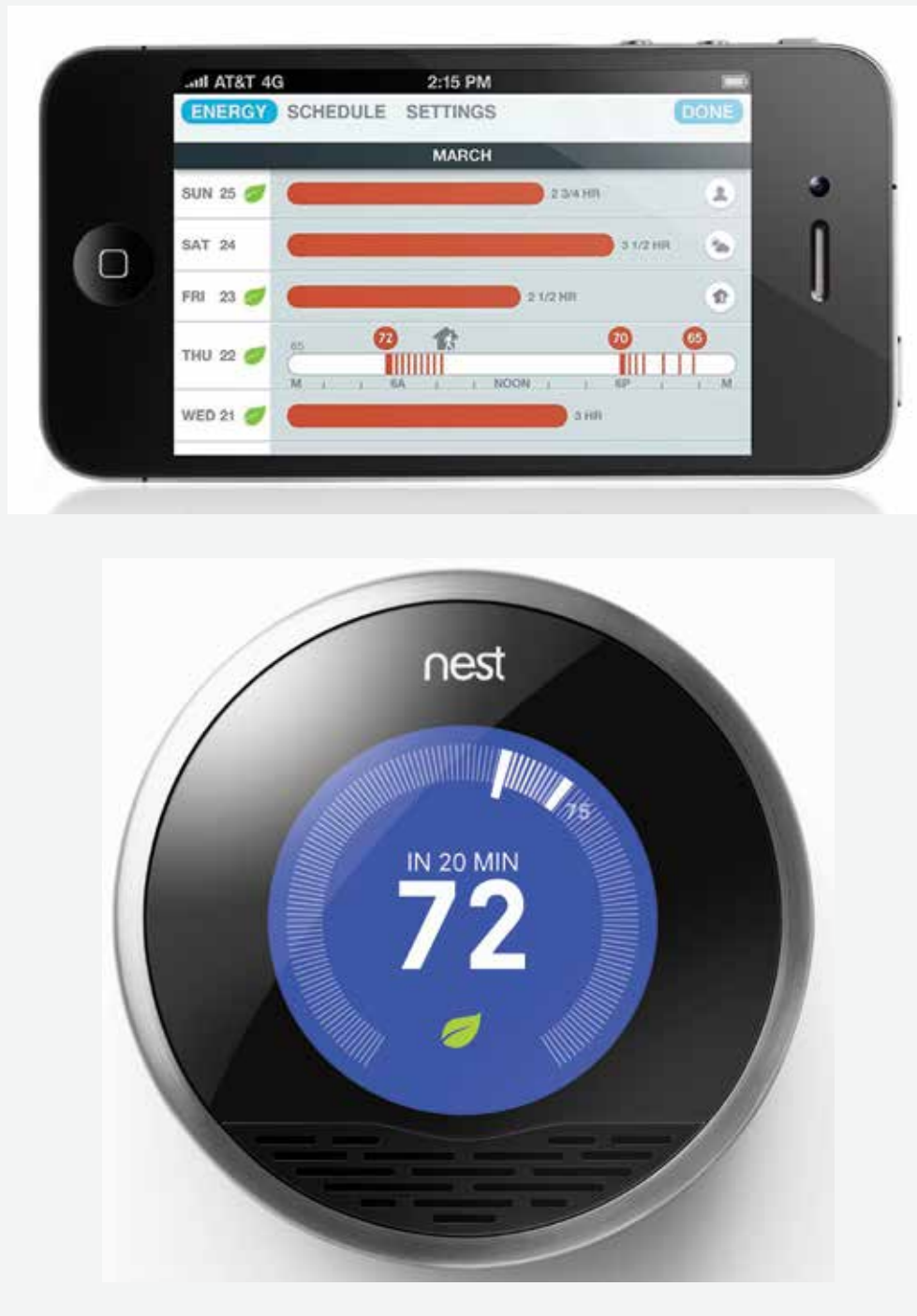
Figure 7: NEST energy system – feedback unit and temperature control wheel
